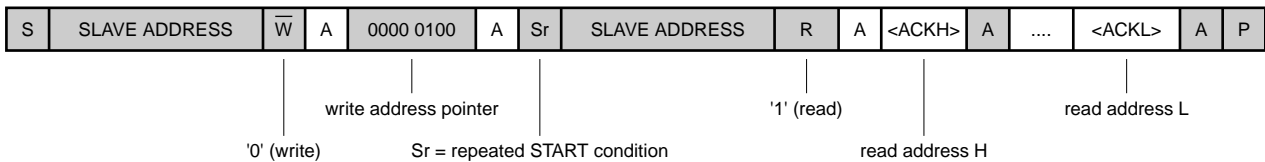
Fig 5. Host reads TDA9951 status register without setting address pointer (pointer was at 0 already)
