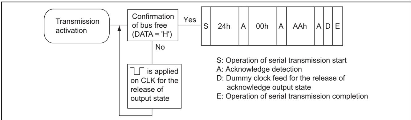
(2) The writing operation of the setting data (FFh, 80h, EEh) into M65667FP internal address of 04h to 06h
