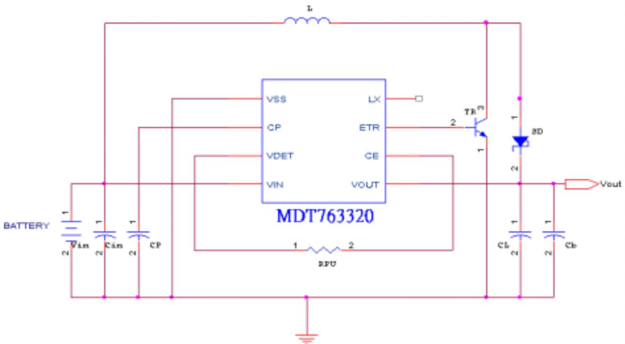
External Transistor application -----using N-Channel Power MOS FET(1A)
