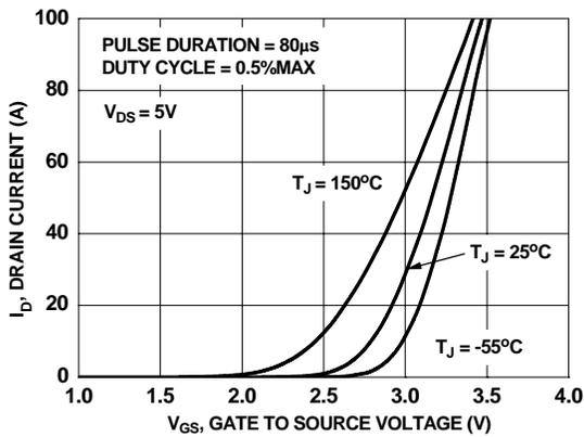
Figure 5. Transfer Characteristics
