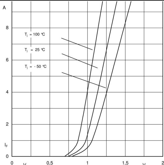
Fig. 1 Forward characteristics (typical values)
