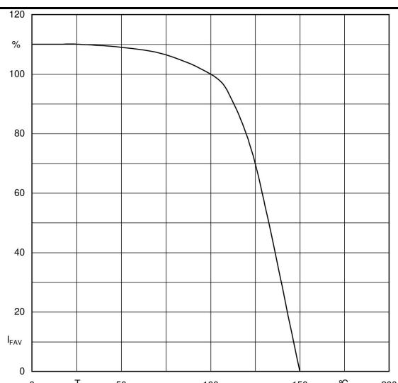
Fig. 2 Rated forward current vs. temp. of the terminals<sup>4)</sup>
