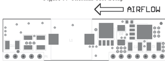
Figure 9. Thermal Test Setup
