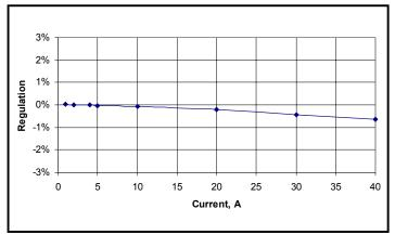
$V_{\text{out}} = 1.1V$
