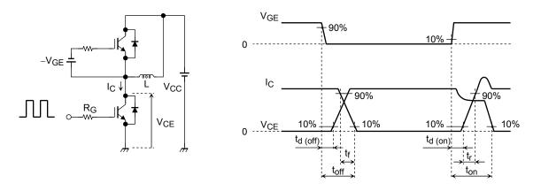
Note 2: Switching loss measurement waveforms
