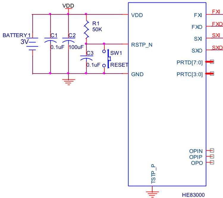
No External Parts is necessary if user adopt Internal Fast RC Clock
