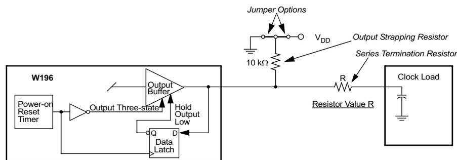
**Figure 2. Input Logic Selection Through Jumper Option**
