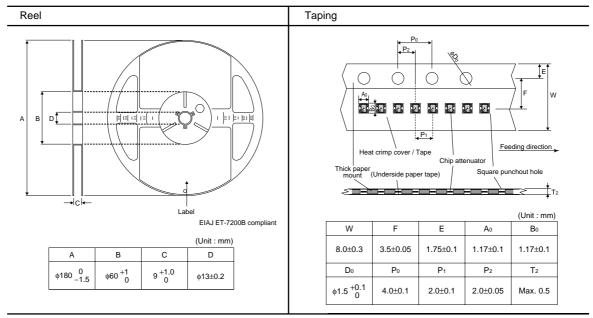
Caution: Insertion direction of device to carrier tape.
