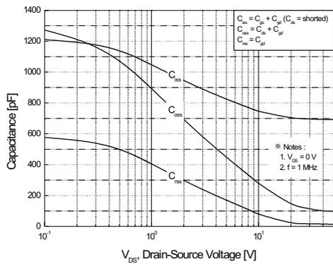
Figure 5. Capacitance Characteristics
