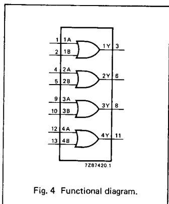
Fig. 4 Functional diagram.
