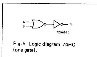
Fig. 5 Logic diagram 74HC
