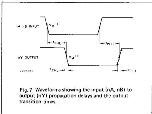
Fig. 7 Waveforms showing the input (nA, nB) to output (nY) propagation delays and the output transition times.
