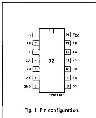
Fig. 1 Pin configuration.
