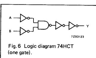
Fig. 6 Logic diagram 74HCT
