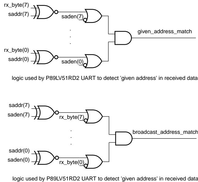
Fig 16. Schemes used by the UART to detect 'given' and 'broadcast' addresses when multiprocessor communications is enabled
