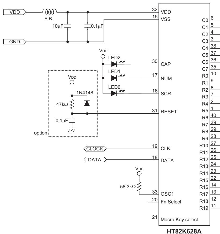
Note: Fn Select → GND: Enable the Mini Keyboard
