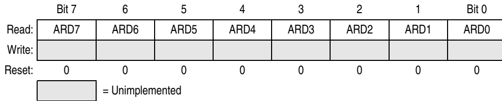
Figure 13-19. ESCI Arbiter Data Register (SCIADAT)
