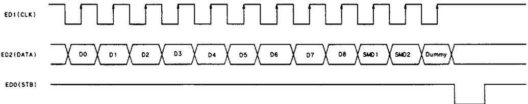
ED2 data is latched to the register at the build up of ED1, and transferred within during the Low period of ED0.
