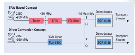
The above figure shows two different tuner concepts for DVB-S/DSS receivers. A satellite dish receives the incoming signal and a LNB converts it to a 1st IF signal. In the SAW based concept the 1st IF signal is converted to  $2^{\rm nd}$  IF by a tuner. Adjacent channels are suppressed by a SAW filter. An I/Q mixer splits up the  $2^{\rm nd}$  IF signal into I and Q components and converts the signals to baseband.
