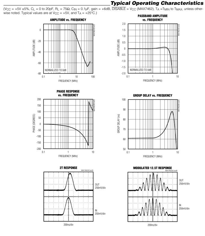
$(V_{CC} = +5V \pm 5\%, C_L = 0 \text{ to } 20\text{pF}, R_L = 75\Omega, C_{IN} = 0.1\mu\text{F}, \text{gain} = +6\text{dB}, \overline{\text{DISABLE}} = V_{CC}$  (MAX7462), T<sub>A</sub> =T<sub>MIN</sub> to T<sub>MAX</sub>, unless other-
