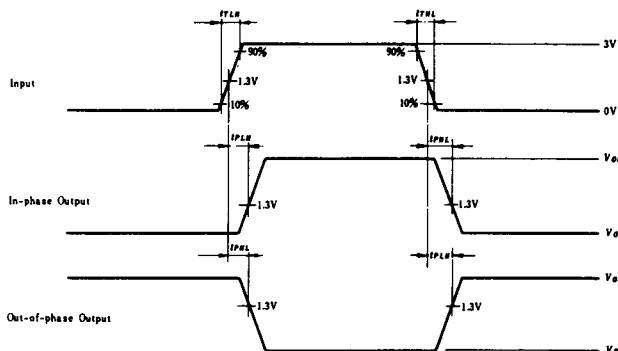
Notes) 1. Input pulse:  $t_{TLH} \leq 15\text{ns}$ ,  $t_{THL} \leq 6\text{ns}$ ,  $PRR=1\text{MHz}$ ,
