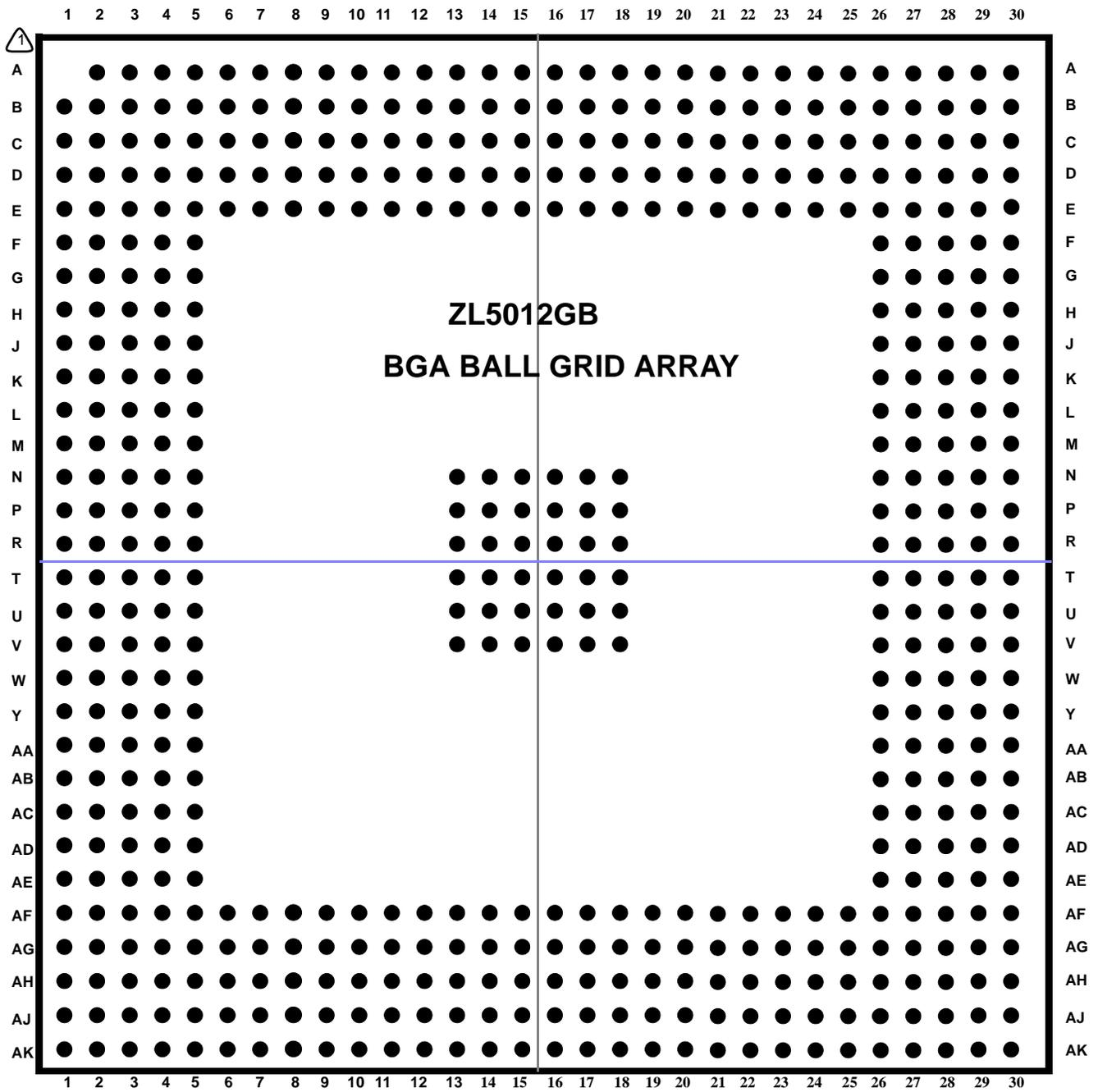
Figure 3 - 535 Ball BGA Ball Grid Array
