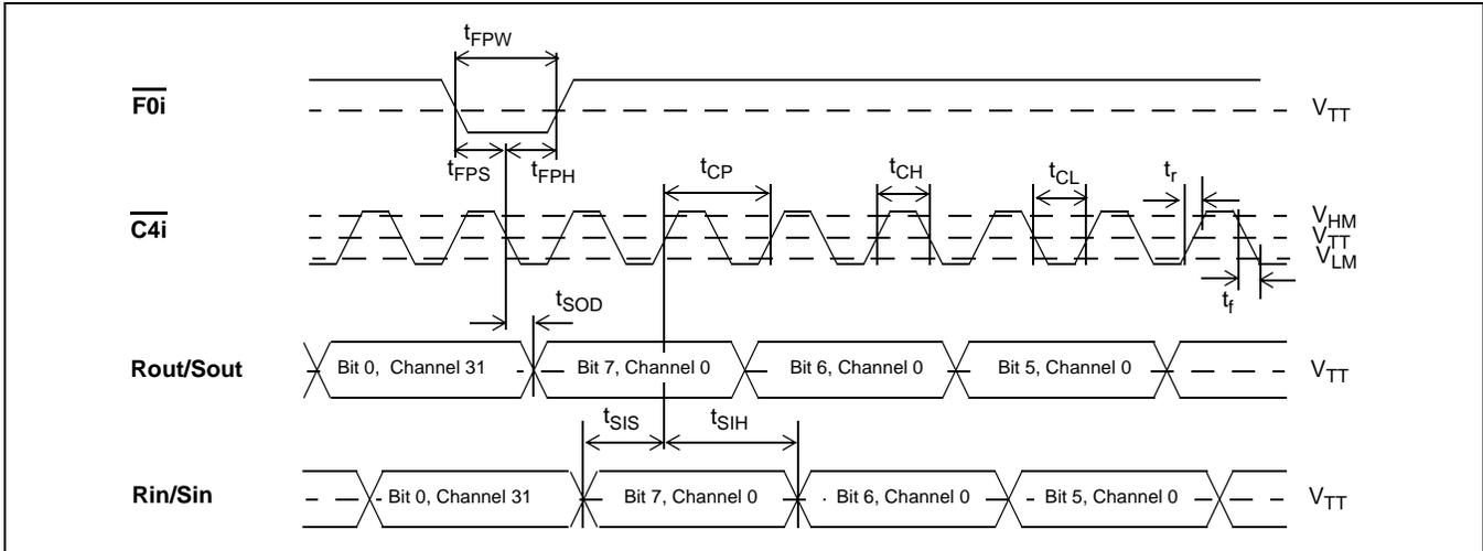
Figure 11 - ST-BUS Timing at 2.048 Mb/s
