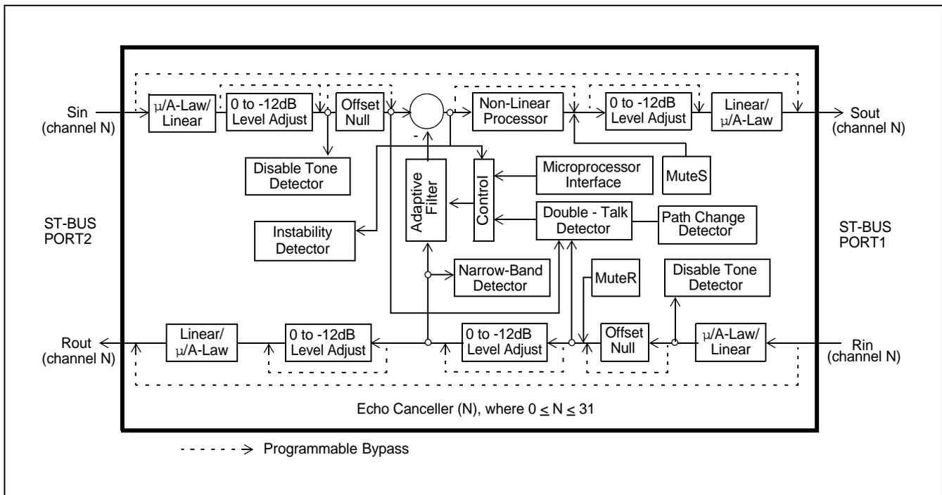
**Figure 4 - Functional Block Diagram of an Echo Canceller**
