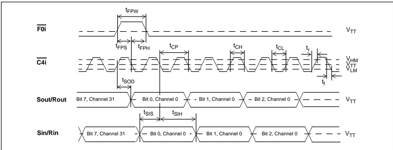
Figure 12 - GCI Interface Timing at 2.048 Mb/s
