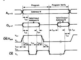
Note: ① 0.1µF capacitor must be connected between  $\overline{\text{OE}}/N_{pP}$  and ground to suppress spurious voltage transients which may damage the device.
