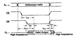
**Notes:**  $\odot$   $\overline{\text{OE}}$  may be delayed up to  $t_{\text{ACC}} - t_{\text{OE}}$  after the falling edge of  $\overline{\text{CE}}$  for read mode without impact on  $t_{\text{ACC}}$ .
