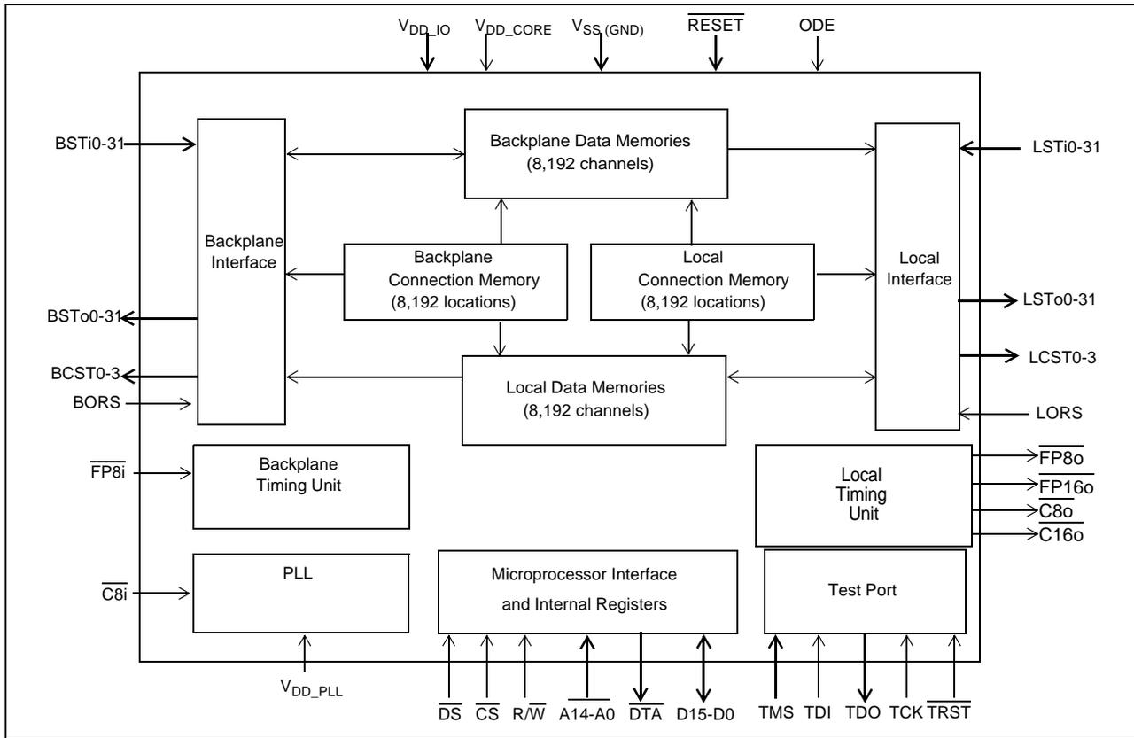
**Figure 1 - MT90869 Functional Block Diagram**
