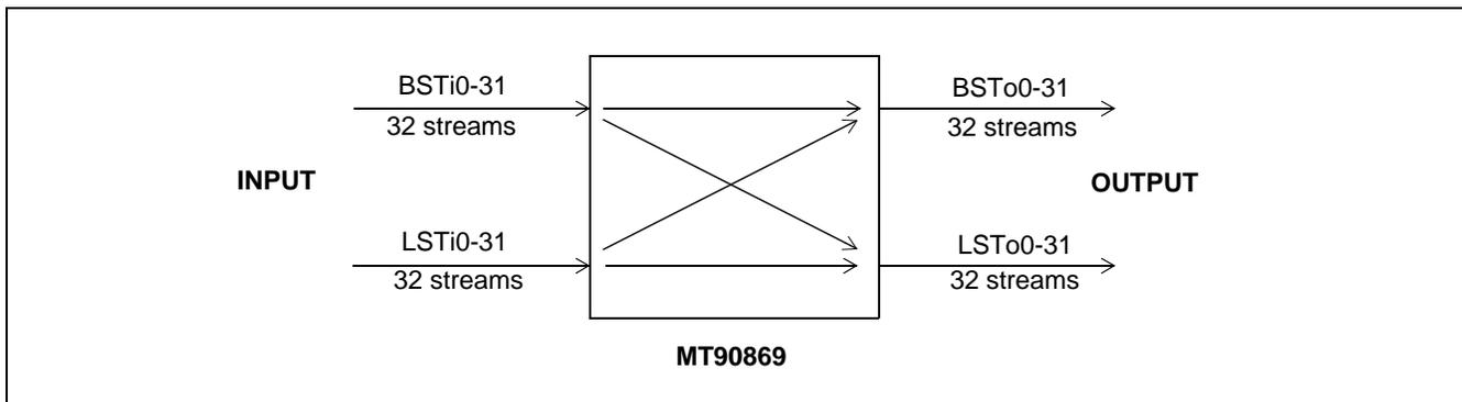
**Figure 4 - 16,384 x 16,384 Channels (16Mb/s), Unidirectional Switching**
