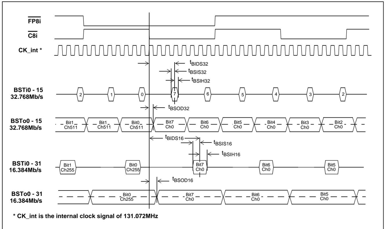
Figure 23 - ST-BUS Backplane Data Timing Diagram (32Mb/s, 16Mb/s)
