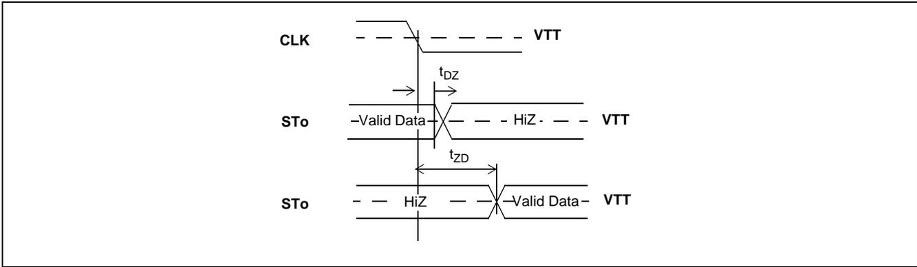
Figure 28 - Serial Output and External Control
