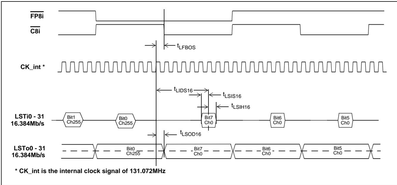
Figure 26 - ST-BUS Local Timing Diagram (16Mb/s)
