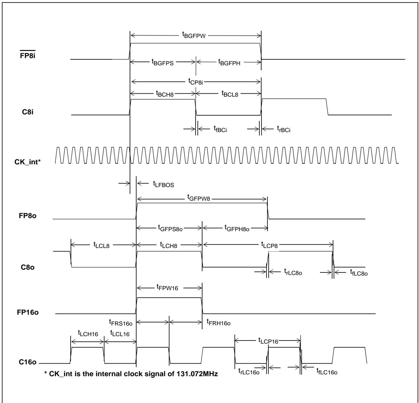
Figure 21 - Backplane and Local Clock Timing for GCI-BUS
