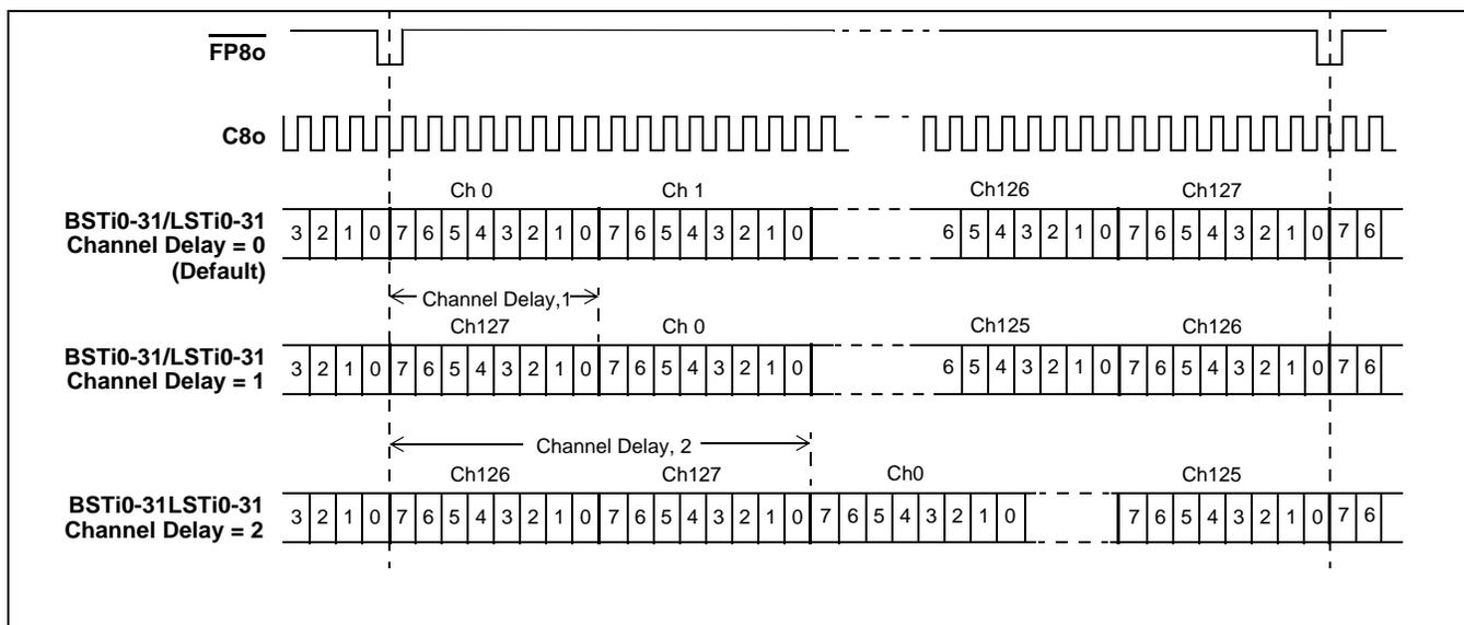
Figure 9 - Backplane and Local Input Channel Delay Timing Diagram
