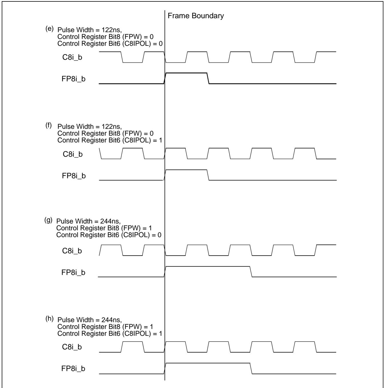
Figure 19 - Frame Boundary Conditions, GCI - BUS Operation
