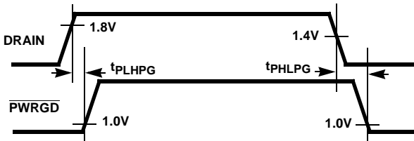
FIGURE 4A. DRAIN TO \overline{\text{PWRGD}} TIMING (ISL6140)
