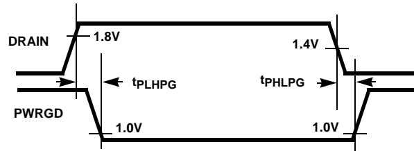
FIGURE 4B. DRAIN TO \overline{\text{PWRGD}} TIMING (ISL6150)
