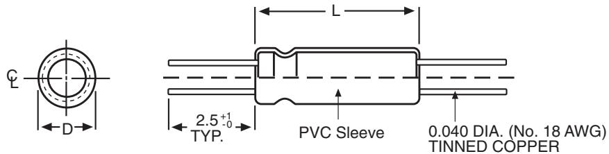
$\frac{0.040}{1.016}$  Diameter (No. 18 AWG) - Case Diameter G,H,J
