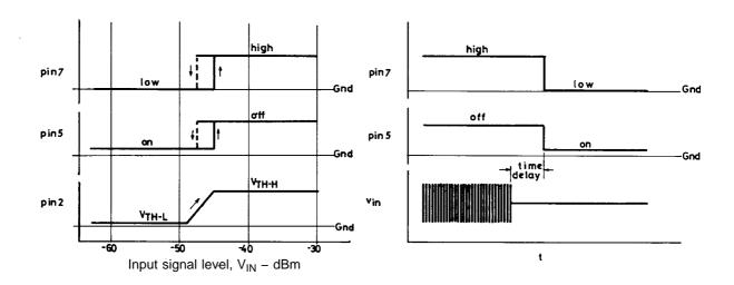
As shown above, when input level is raised and the pin 2 voltage reaches the  $V_{TH-H}$  level of the comparator, pins 5 and 7 turn over. ( $V_{IN} = -45 \text{ dBm}$ ).
