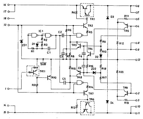
· Since pin 12 is grounded to the substrate, noise may be affected when a heat sink is connected to the FG (Frame Ground), GND line, etc.
